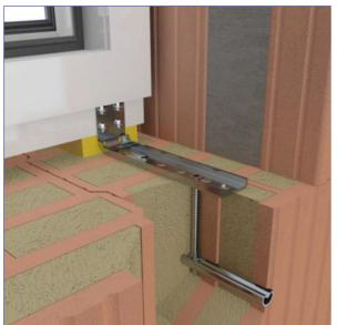
For secure window mounting on the vertically perforated brick with big chambers.
