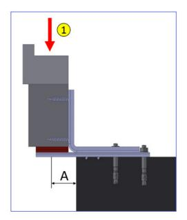
For secure mounting underneath floor-depth elements Right-angled bracing of the balcony connection profile Offers high load transference Simple and fast mounting in case of an already existing insulating layer Maximum load tested by ift-Rosenheim Suitable for fall-proof window mounting
